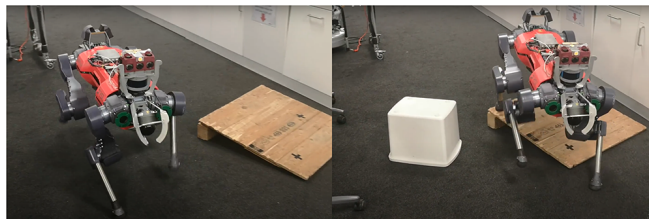
Fig. 10. The navigation framework prefers flat ground than the low-lying obstacle, while if other ways are blocked, it can also navigate the robot to walk across the obstacle.
