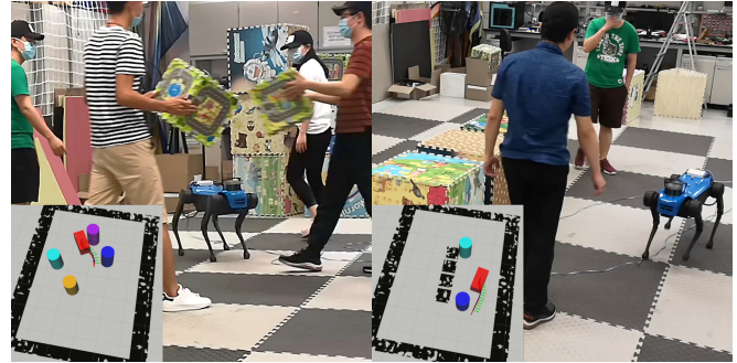
Fig. 1: The proposed local planner performs online interaction estimation with mobile agents and the static environment, providing efficient and cooperative crowd navigation solutions that fully utilize the agile motion capabilities of quadrupedal robots in highly dynamic scenarios.
